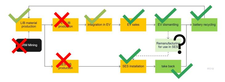
Next to material recycling, LIB from EV have potential to be remanufactured into stationary energy storage (SES)
